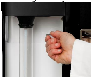
Fig. 10. Closing the Protection door and starting a distillation
