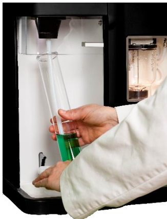
Fig. 9. Inserting a tube in the KjelROC Distillation Unit
