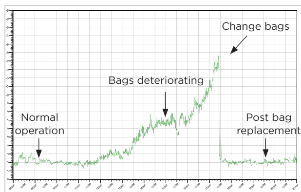
Figure 2: PCME LEAK ALERT 73 monitoring bag-leak conditions
