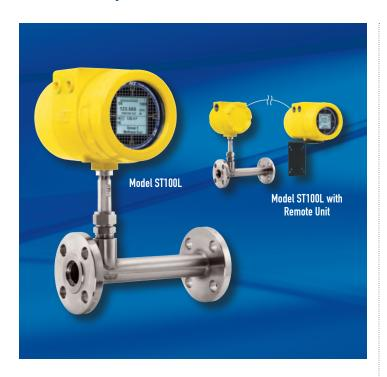
The Model ST100L is an in-line, spool piece gas flow meter that combines best-in-class transmitter/electronics and superior calibration to provide a truly state-of-the-art gas flow meter for industrial process and plant applications with line sizes up to 2 inches [50 mm].
